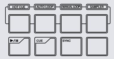
The performance pads have eight different modes you can select. The first four modes are; Hot Cue Mode (1-4), Auto Loop Mode, Manual Loop Mode and Sampler Mode.
